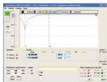
Fig. 14: A commercial v.h.f. notch filter gives a dip (tunable) of around -28dB at 87MHz and a poorer -18dB at 170+MHz.
