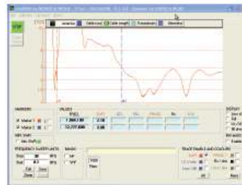
Fig. 2: The s.w.r. plot of my end-fed 65J antenna with its 20m long element.
